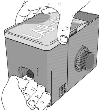
Push the grey lever upwards on the back to release the film from the cartridge.
